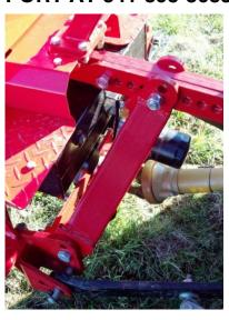
\* Most people will raise the lower 3-Point hitch arm to a lever position and then adjust the main frame to vertical. This is fine and is the best position for safe transport, however the lower or closer the backhoe is to the ground the deeper it can dig.
