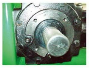
After 50 hr of work, check and fill the gearbox to the required level, using oil type SAE 90 EP API GL4 Oil.
