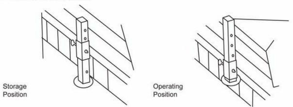
In order to keep the machine stable, lower the adjustment stand when the machine is stopped (see above drawing).
