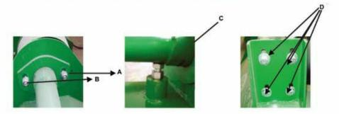
Adjust the drive belt tension. The correct belt tension is achieved when the belt can be deflected by the belt thickness about 10mm at the center point between the pulleys.
